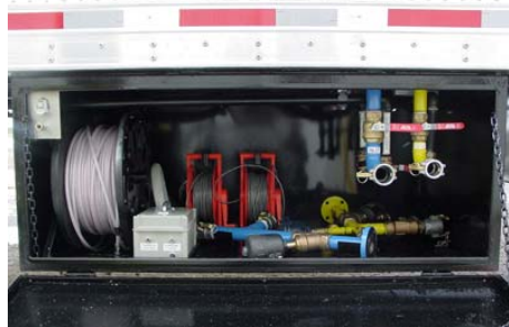
Level Monitor Assembly & Required Hose Reels(For Pneumatic and Electrical Connection of Remote Level Monitor Assembly)
